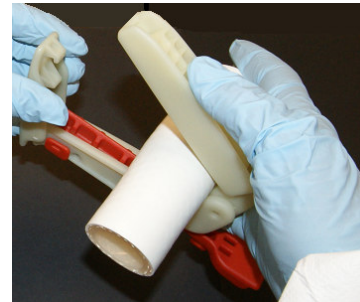
7. The Lower-Member is free rotate it up and rearward
