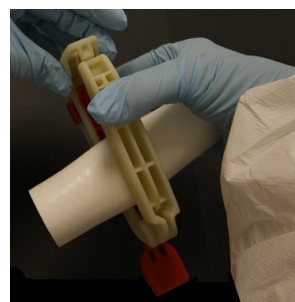
6. Pull the Locking-Link from the Lower-Member
